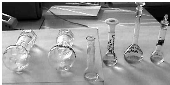
Fig. 2 Sample Aliquat 336 ® -based ILs. From left to right: [A336][HCO 3 ], [A336][H 2 PO 4 ], [A336][Cl] (neat Aliquat 336 ® ), [A336][HSO 4 ], [A336][NO 3 ] and [A336][OCN] (from NaOCN).
